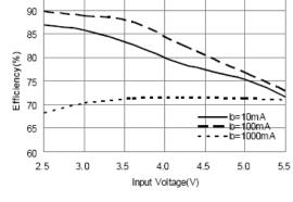
Efficiency vs Input Voltage (Vo=1.2V)
